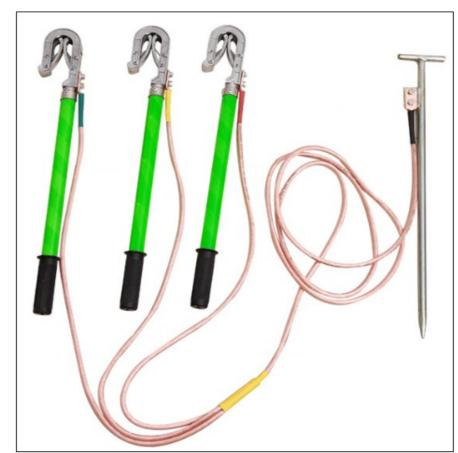
Ground (grounding) sticks allow current-carrying conductors to be intentionally bonded to one another and grounded to earth while they are deenergized to act as a safety precaution should the conductor(s) be unintentionally re-energized.
