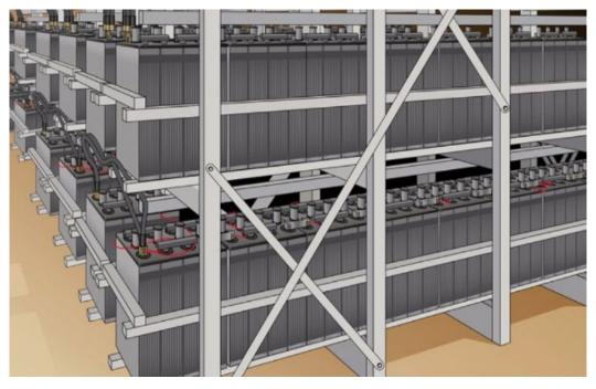
Battery maintenance involves checking cable termination torque to prevent loose connections from expanding and contracting metals and cleaning corrosion from terminals as needed.
