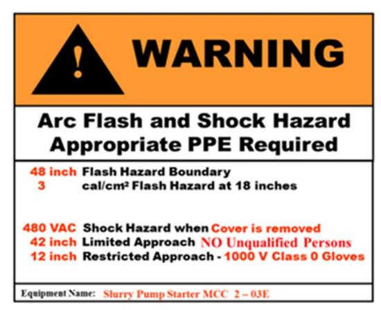
This equipment label warns workers that a flash hazard boundary exists within 48 inches of the equipment.
