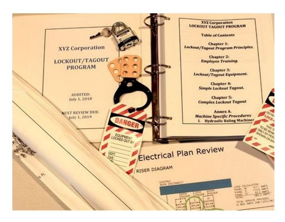
The lockout/tagout program must specify the procedures to protect workers from electrical hazards.
