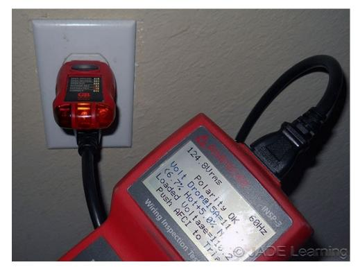
Test instrument power cords are addressed in Section 110.7 (A) and (B).
