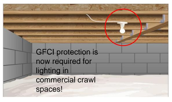
Don't forget: All **GFCI** devices must be readily accessible.
