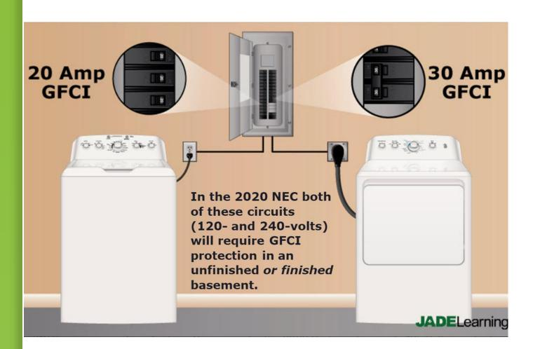
In the 2020 NEC dwelling unit receptacles up to 250-volts (not until 1-01-2022 for lowa) require GFCI protection in 11 locations specified in NEC Section 210.8.
