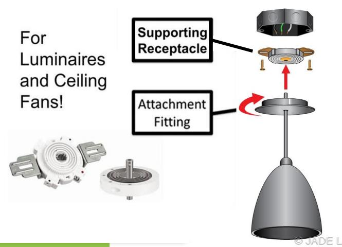
A device that, by insertion into a locking support and mounting receptacle, establishes a connection between conductors of the attached utilization equipment and the branchcircuit conductors connected to the locking support and mounting receptacle.
