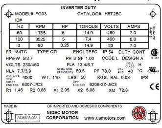
This motor will be controlled by a VFD
