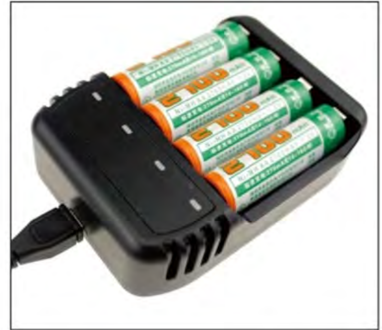
Batteries act as electrolytic cells during charging.
