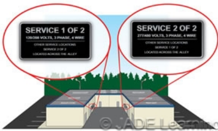
Separate services must be individually identified.
