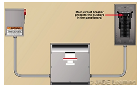
The overcurrent protection for a panelboard that is supplied from a transformer on the secondary side of a transformer must protect the panelboard busbars and the transformer secondary conductors.
