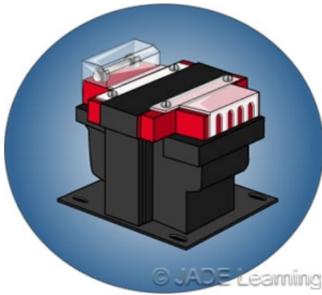
A motor control circuit transformer must have overcurrent protection.
