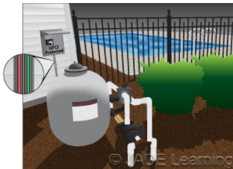
Different types of wiring methods are permitted in corrosive and noncorrosive areas around swimming pools.
