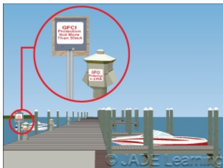
GFCI protection with trip settings at 30 mA are required for overcurrent protective devices that supply residential docking facilities.
