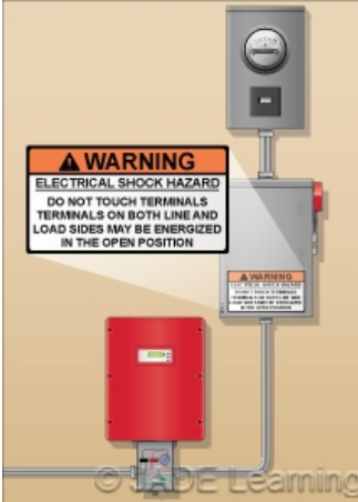
A warning sign is required for all power source disconnects that may be energized from both directions.
