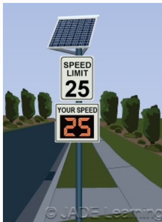
A stand-alone system operates independently of the utility grid.
