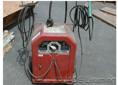
Arc welders are a common example of cord-and-plug equipment that must be grounded.
