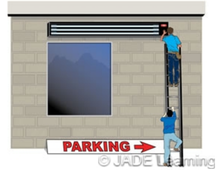
Non-current-carrying metal parts of signs and outline lighting are required to be grounded.
