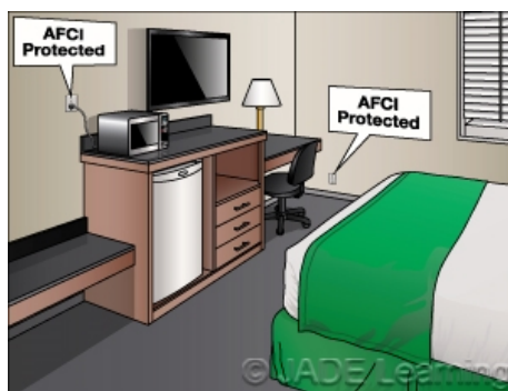
All 15- and 20-amp rated branch circuits supplying guest rooms and guest suites, with or without permanent provisions for cooking, are required to have AFCI protection.
