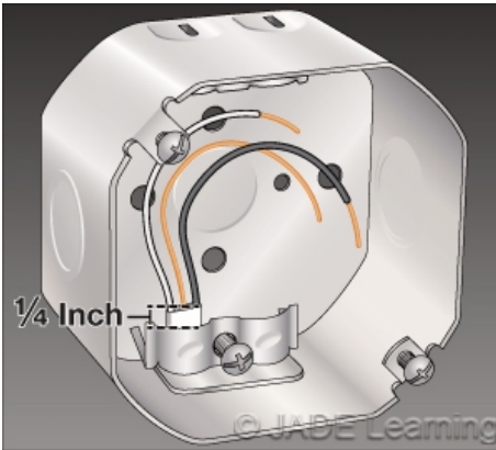
The sheaths of nonmetallic cable must extend at least 1/4 inch into a metal box and beyond any cable clamp.
